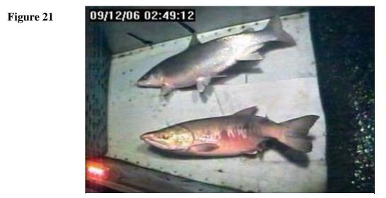
Infrared triggered LED testing light going on as fish pass sensor in slot mid chute (by sheefish dorsal fin).
