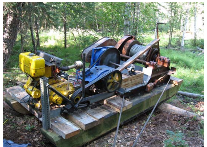
Winch used by project to pull wheel out of water at Rapids
