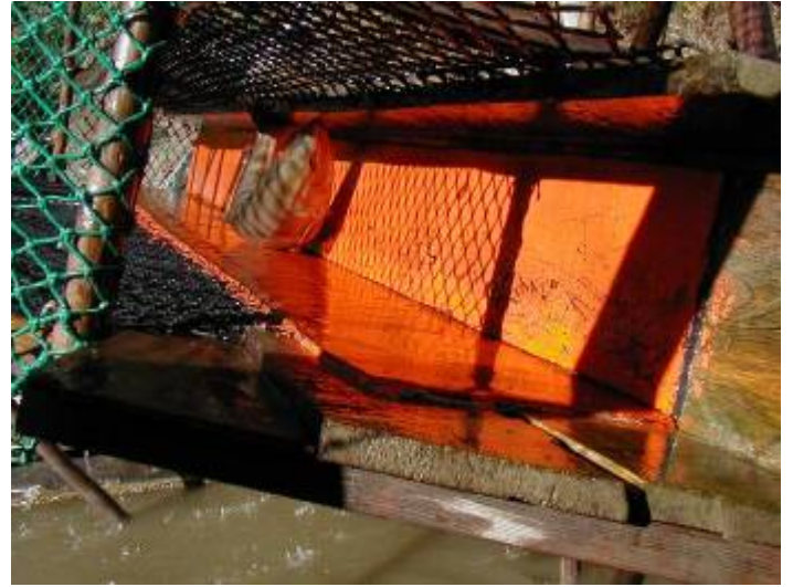
Strategic placement of closed cell foam padding reduces injury dramatically to the fish.
