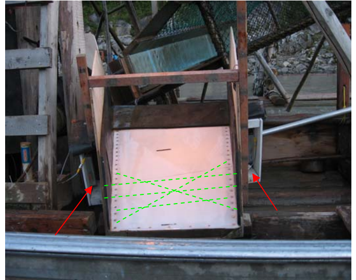
Infrared transmitter / receiver placement (red), and general direction of beams across chute (green).
