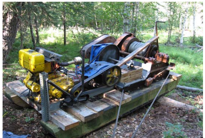
Winch used by project to pull wheel out of water at Rapids in 2010
