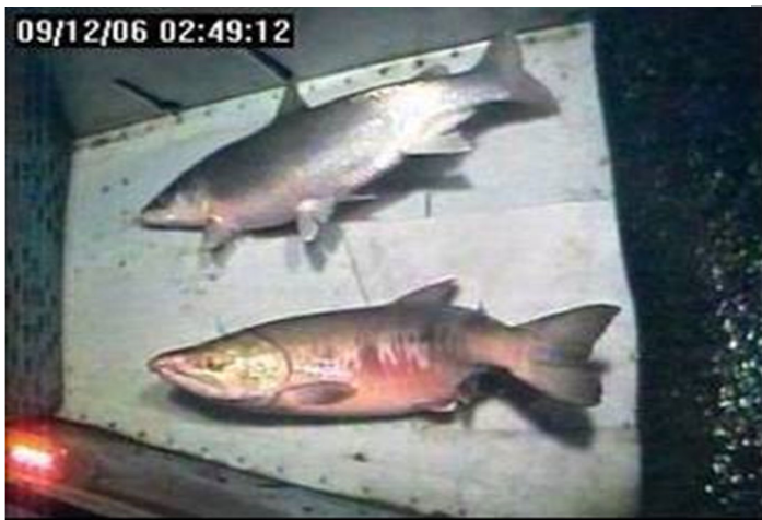
Infrared triggered LED testing light going on as fish pass sensor in slot mid chute (by sheefish)
