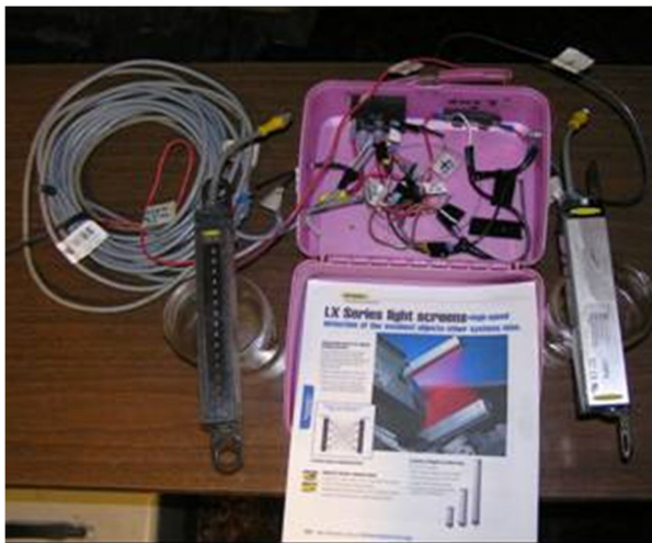
Infrared transmit and receive arrays and control lunchbox
