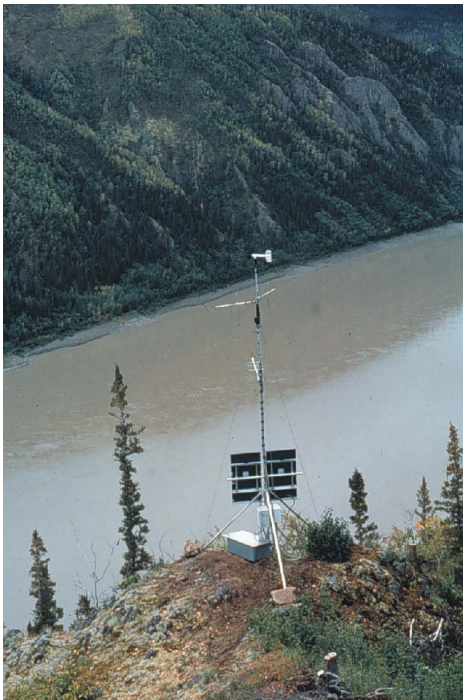
FIGURE 16.—Remote radio receiving station located on a high bluff over the Yukon River, 11 km upstream of the study site. This station, and others like it, recorded the passage of radio-tagged inconnu moving along the river.
