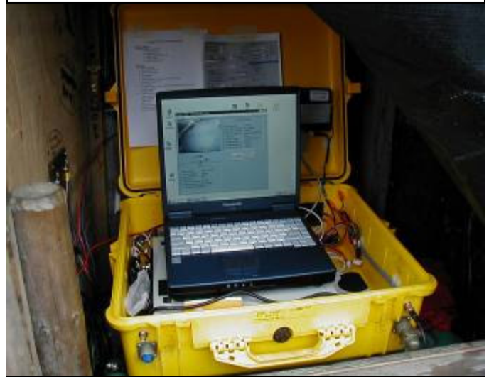
Compact laptop/VCR capture system for Fishwheel installation.
