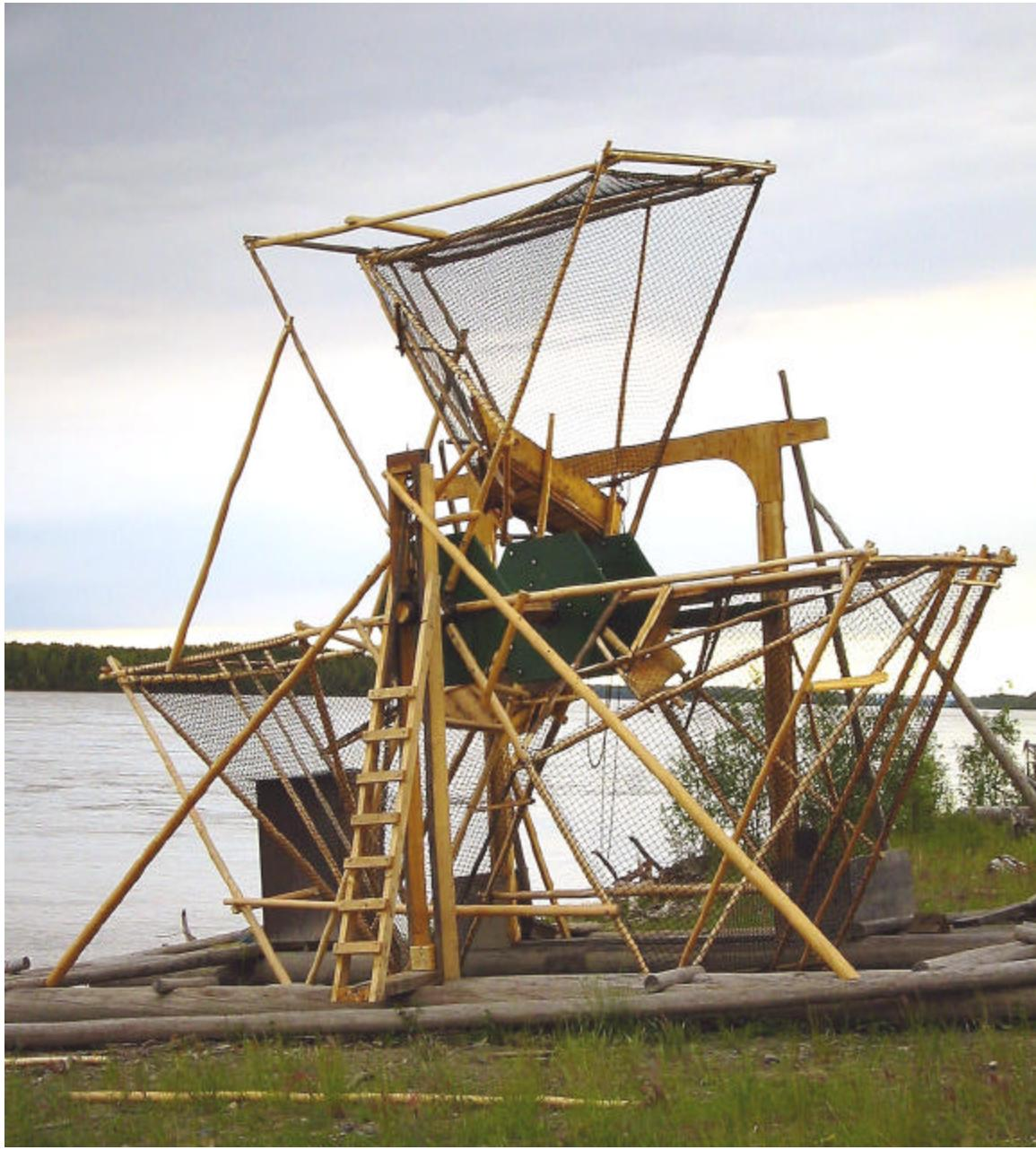
A new fishwheel was built in 2002 using features and materials that are ‘softer’ on salmon; the design also provided a more consistent rotation speed than the old design. The fishwheel is hexagonal with 3 baskets mounted 120 degrees apart.
