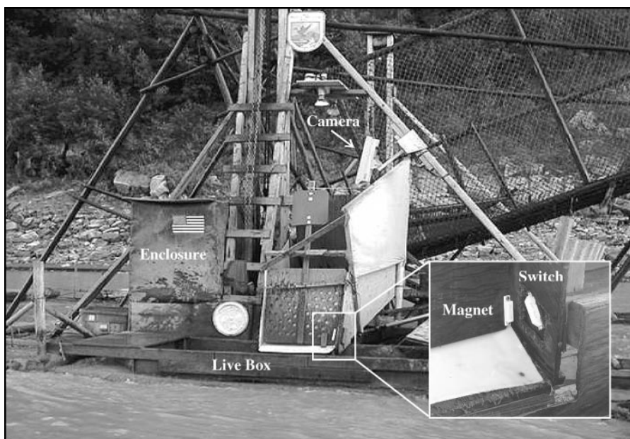
FIGURE 1.—Switch-triggered video system installed on a Yukon River fish wheel. The magnet and switch are shown enlarged in the inset. The enclosure housed a notebook computer, time-lapse videocassette recorder, fuse box, and 12-V battery bank.
